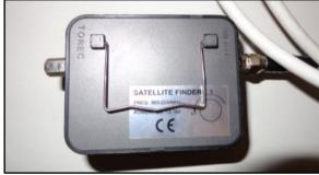
Figure 12 - SAT FINDER with jumper cable
