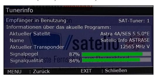
Figure 14 - Signal Level Indicator
